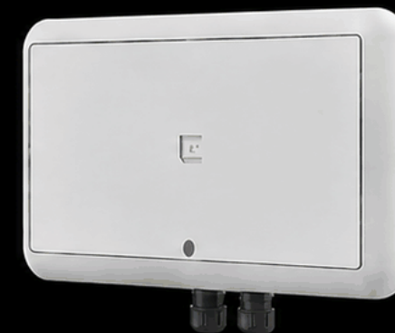
AP5060D — Directional Access Point Configurable beamwidth: 20° or 70°
